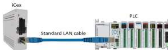
Fig. 1 Connect direct iCex to device (PLC) via Ethernet
